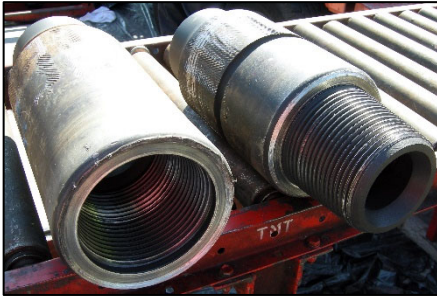
Example of seal face and thread damage
