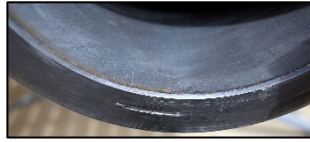
Example of seal face cut & protrusion
