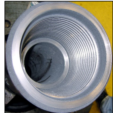
Example of clean threads & refaced shoulders
