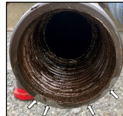
Seal face damage from Top Drive sub
