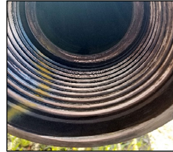
Example of stabbing damage on the seal face
