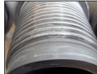
Example of first few threads stabbing damage
